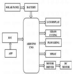
Fig 9: Block diagram
